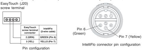
8. Insert the screw terminal onto the EasyTouch **COM-PORT** (**J20**) board connector. *Note: Multiple wires may be inserted into a single screw terminal.*
